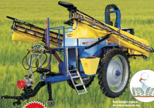
Y-3 / 2400 Lt. Hava Destekli Tarla Pülverizatörü Y-3 / 2400 Lt. Air Supported Field Sprayer (Y-3 / 2400 Lt. Air Supported Field Sprayer)
